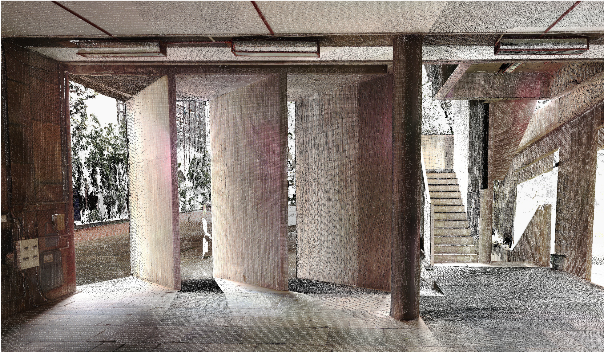
View generated from the 3D point cloud model of ATMA House, Ahmedabad. Data collected by workshop participants under the guidance of M. Mane, Z. Pithawalla, SreeRam. Post processing and visualization by M. Mane, Z. Pithawalla, and SreeRam for CHC - CRDF.
