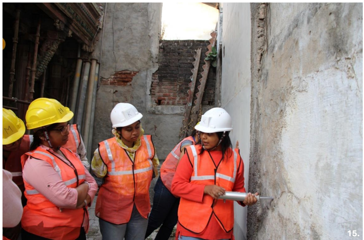
Image 13: CPP participant taking a reading from the moisture meter at Mukhi Delu.
