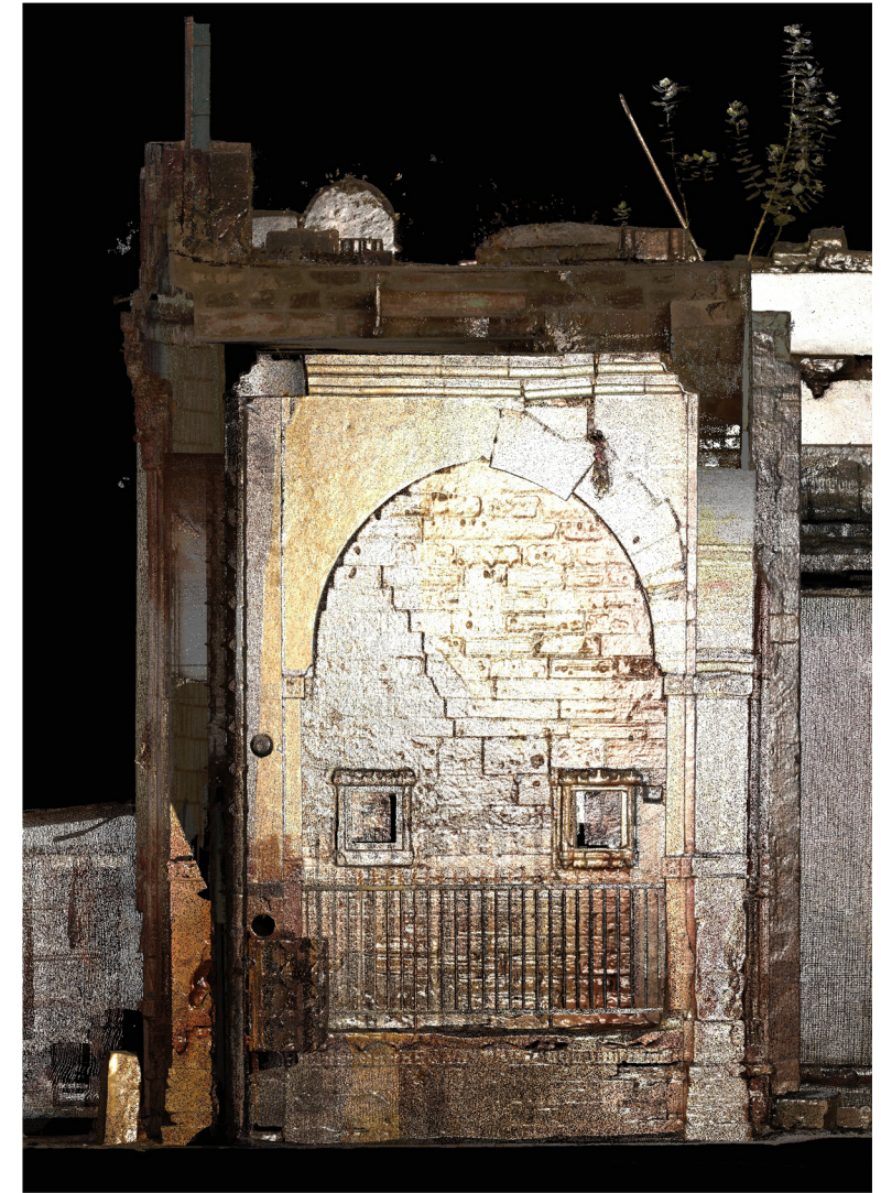
Sectional view generated from the 3D point cloud model of Nagarkhana, Darbargadh, Kutch. Data collected by workshop participants under the guidance of M. Mane, Z. Pithawalla, D. Nakrani. Post processing and Visualization by M. Mane, Z. Pithawalla, and D. Nakrani for CHC - CRDF
