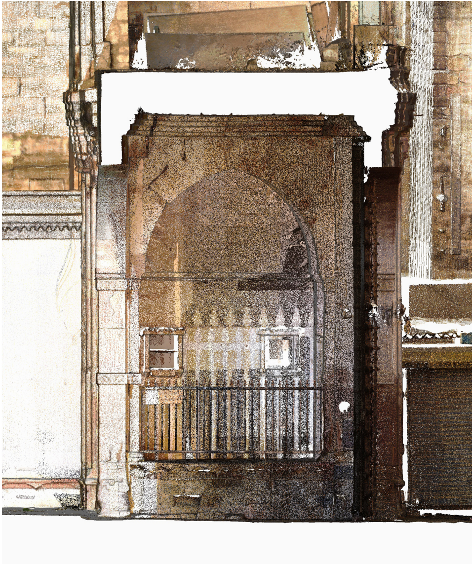
Sectional view generated from the 3D point cloud model of Nagarkhana, Darbargadh, Kutch by V. Purohit as part of MCR 2021, CEPT University. Data collected by workshop participants under the guidance of M. Mane, Z. Pithawalla, D. Nakrani. Post processing and Visualization by M. Mane, Z. Pithawalla, and D. Nakrani for CHC - CRDF.
