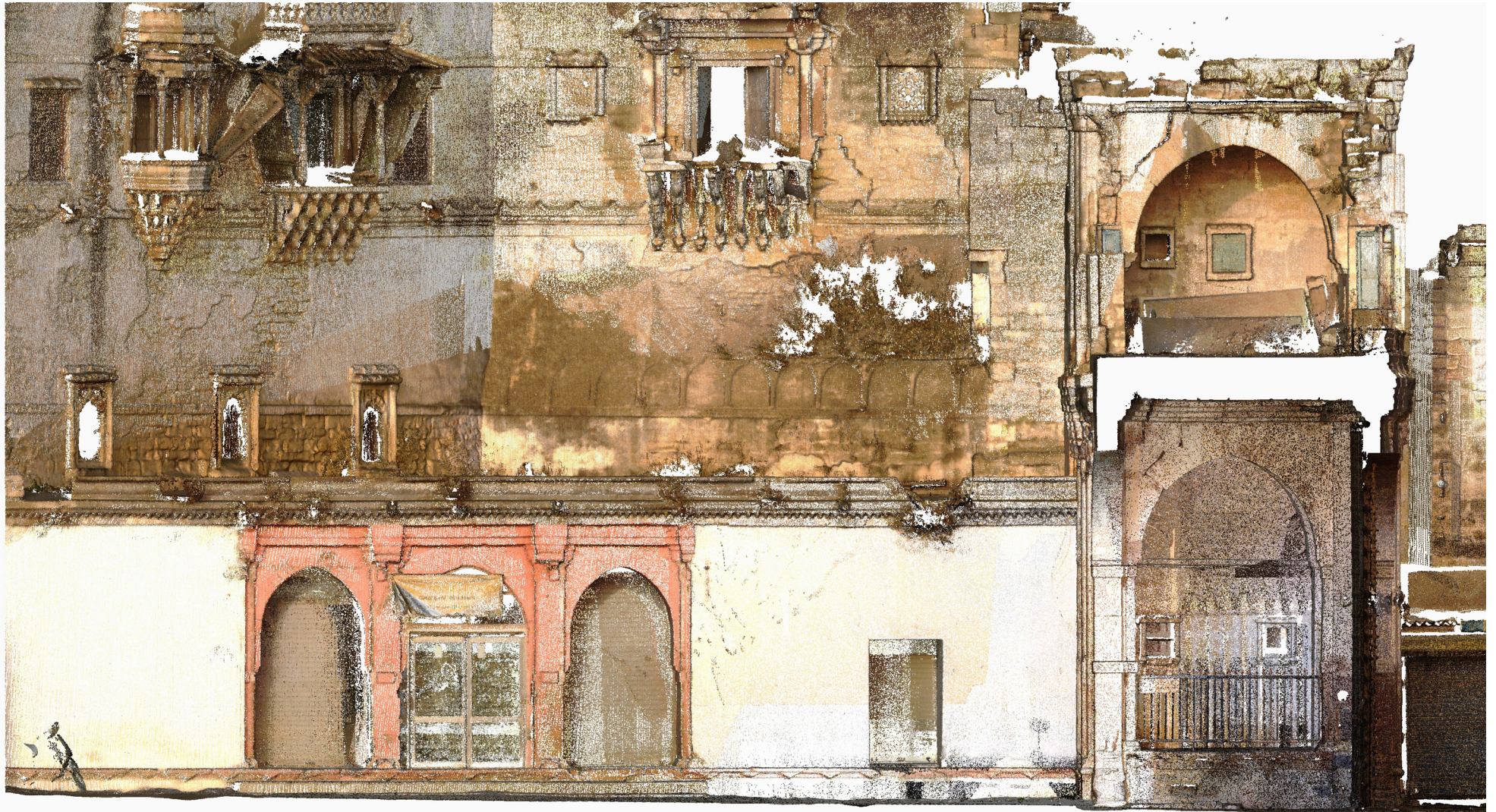
Sectional view generated from the 3D point cloud model of Nagarkhana, Darbargadh, Kutch by V. Purohit as part of MCR 2021, CEPT University. Data collected by workshop participants under the guidance of M. Mane, Z. Pithawalla, D. Nakrani. Post processing and Visualization by M. Mane, Z. Pithawalla, and D. Nakrani for CHC - CRDF.
