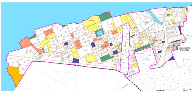
Figure 15: T P Scheme delineated based on a physical feature (Sabarmati River)- Source: TPVD, Govt. of Gujarat
