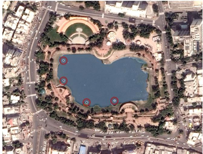
Figure 54 : Networking storm water drains to rain water recharge wells in Vastrapur lake- a case of good practice
