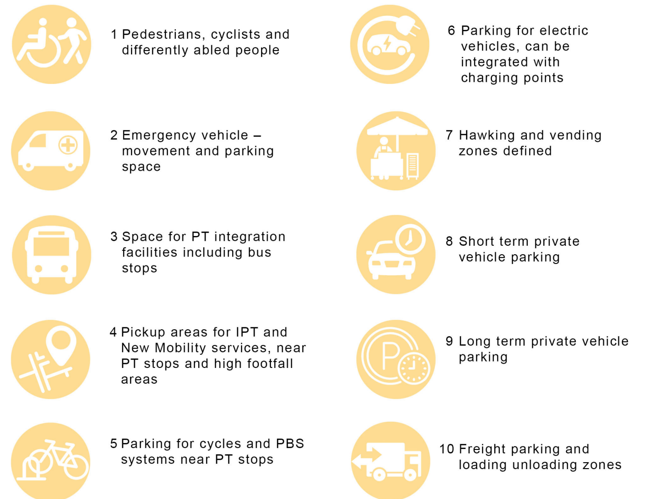
Figure 3: Road space (RoW) usage priority
